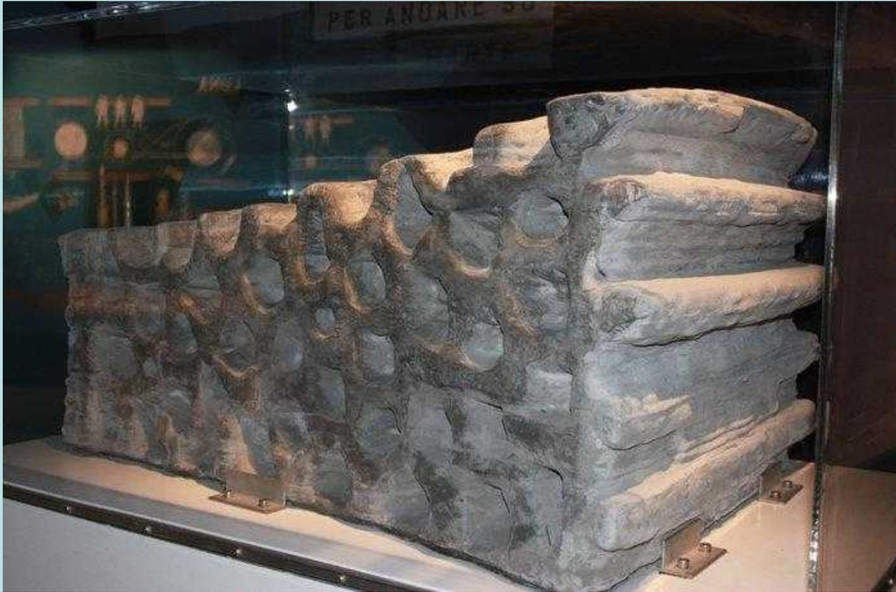
This picture shows a 1.5 tonne ‘Lego brick’ made from a ‘Moon Dust Substitute’. This type of building block could be the basis for a permanent solid moon base. In addition, being made of volcanic silicates it is ~40% Oxygen and therefore a possible source of this gas for lunarnauts/lunatics. 3-D printing could be the technology used to assemble walls and roof from dust. ESA astronaut Samantha Cristoforetti is in charge of the programme, called “Spaceship EAC”.
