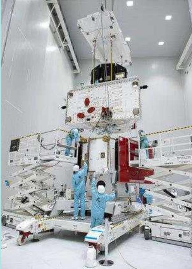
The two science orbiters of the joint ESA-JAXA **BepiColombo** mission are now connected in their launch configuration and the European science orbiter and transport module have been given the go-ahead to be loaded with propellants.
