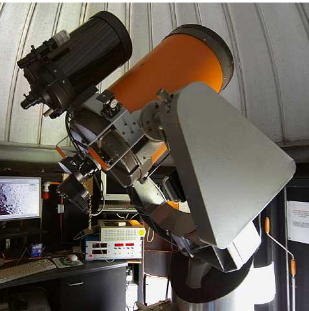
The 14-inch. The handles and sheet-metal covers on the fork, and the piggy-back support for the 8-inch, were fitted by the university.
